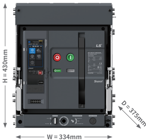
D-Frame ~ 2000AF 50kA @900VAC 30kA @1150V
